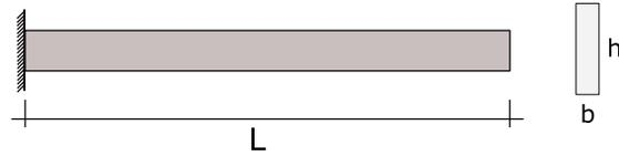
Figure 4: Cantilever beam and cross section for the free vibration problem
