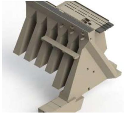
Figure 1: Tridimensional CAD model of a section of the Itaipu dam, Brazil, retrieved from the original documentation [13]
