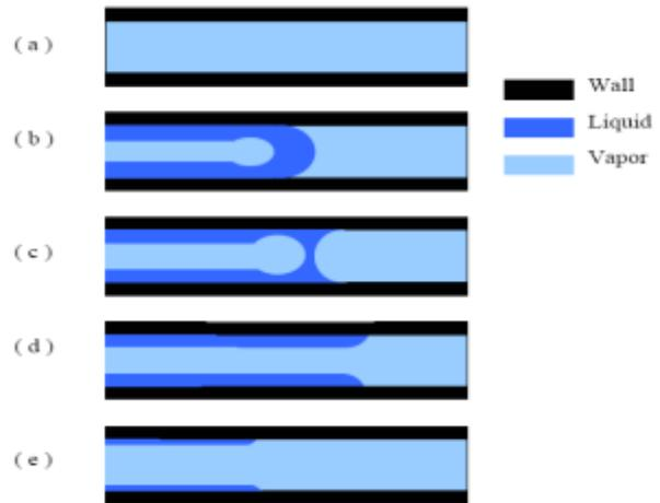
Figure 6. Annular to CHF in Schematic Form. (a) channel dry-out, (b) annular slug with liquid head, (c) contact angle shift, (d) vapor penetration at CHF occurrence, (e) thinning film as it returns to dry-out
