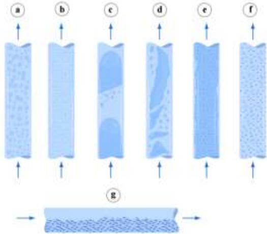
**Figure 7.** Typical configuration of (a) bubbly flow, (b) dispersed bubbly (i.e. fine bubbles dispersed in the continuous liquid phase), (c) plug/slug flow, (d) churn flow, (e) annular flow, (f) mist flow (i.e. fine droplets dispersed in the continuous vapor phase) and (g) stratified flow. Note: mist flow is possible only in a heated channel; stratified flow is possible only in a horizontal channel.
