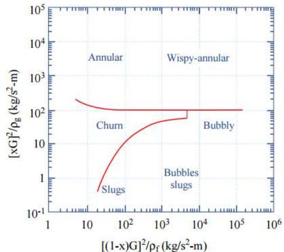
**Figure 11.** A typical flow map obtained from data for low-pressure air-water mixtures and high-pressure water-steam mixtures in small (1-3 cm ID) adiabatic tubes
