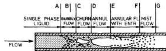
**Figure 1.** Schematic of the vertical flow boiling process.
