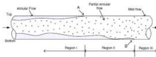
Figure 2. Shear stress distribution in horizontal annular flow.
