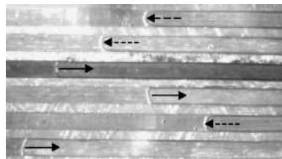
**Figure 8.** Schematic representation of evaporation momentum and surface tension forces on an evaporating interface in a microchannel.
