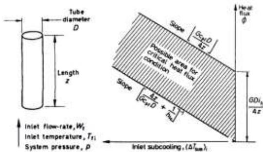
**Figure 12.** Independent variables affecting the critical heat flux for uniformly heated vertical round ducts and the limits of the critical heat flux condition.
