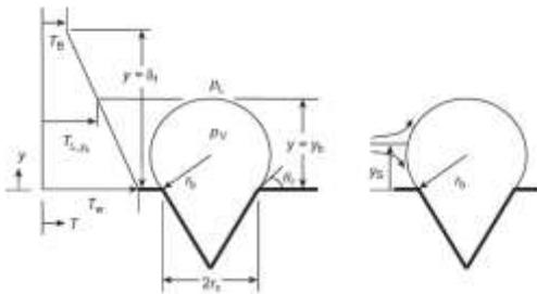
Figure 5. Heat transfer mechanisms of boiling in micro-channels
