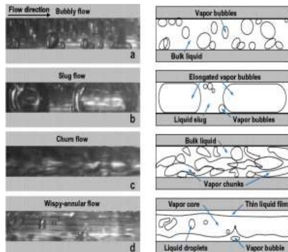
Figure 4. Flow boiling regimes in micro-channels
