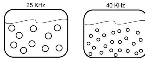
**Figure 1.** Representation of bubbles of cavitation in ultrasound system, illustrating that the 25 KHz (left) the bubbles of cavitation are larger and therefore with low penetration power and 40 KHz (right) bubbles with less volume characterizing with high penetration power.
