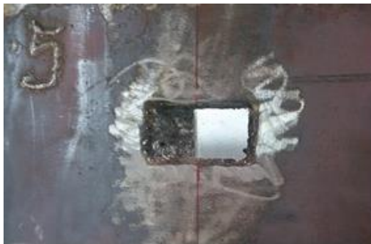
Fig. 3. Cladded and polished sample
