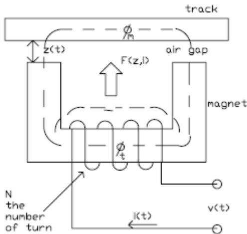
Fig 1 Schematic of an electromagnetic suspension system
