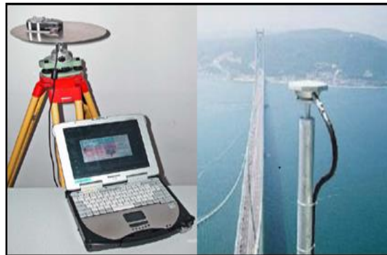
Figure 5. GPS technology, of geodesic rank can be used for monitoring bridges. (Source: Leica)
