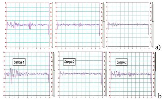
Figure 6. Experimental results from ultrasound scanning of overlaid samples with longitudinal waves: a) sample 4; b) samples 1, 2, and 3.
