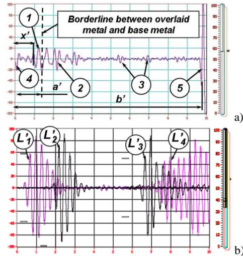
Figure 5. Characteristic results from ultrasound scanning of test samples; a) using longitudinal waves; b) using surface waves.
