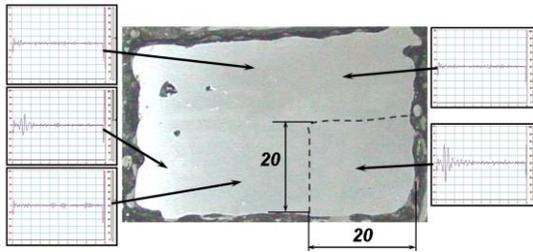
Figure 7. Experimental results from ultrasound scanning of sample 5 with longitudinal waves.
