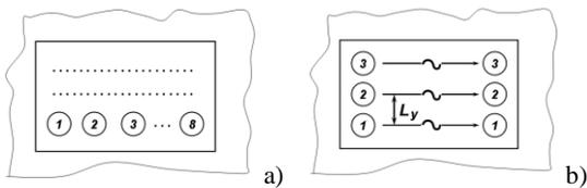
Figure 4. Scheme for carrying out the experiments for scanning with longitudinal waves (a) and taking into account the width of the signal spectrum of the surface wave (b).
