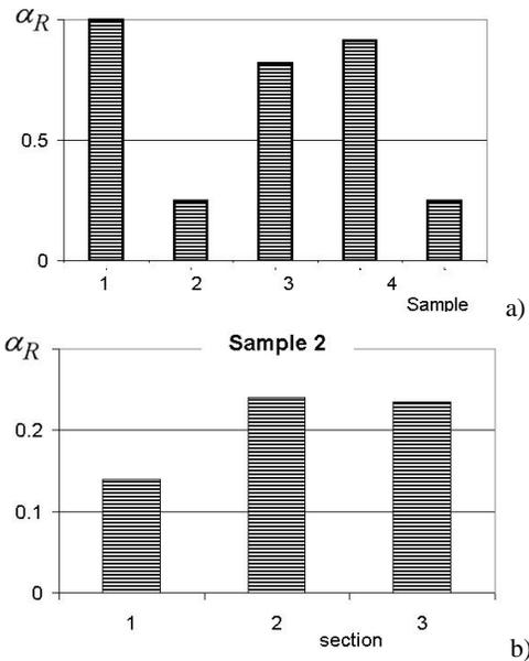
Figure 8. Results for the damping factor  $\alpha$  of the surface wave at  $\Delta L_x = 15\text{mm}$ .
