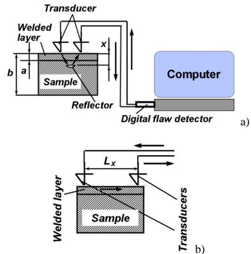
Figure 3. Experimental set-up for ultrasonic examination of the weld layer: a) using longitudinal waves; b) using surface waves.
