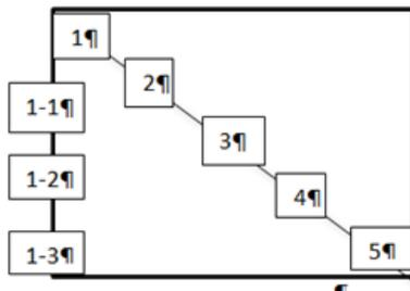
Figure 1. Diagram of the points for Vickers hardness measurement of the samples.
