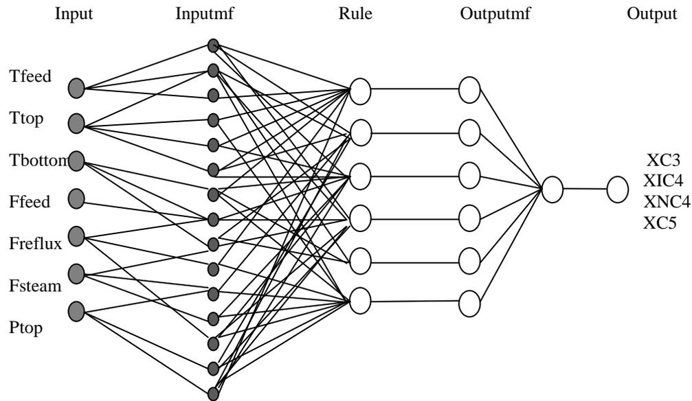
Tfeed = feed temperature      Ttop & Tbottom= top and bottom temperature of debutanizer
