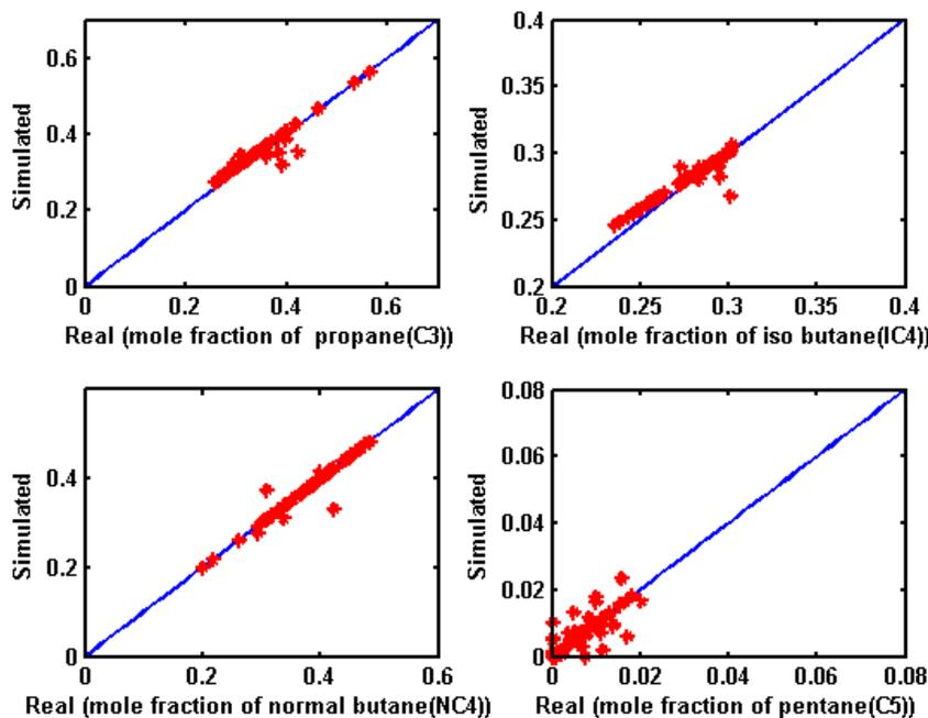
Figure 6. Real vs. simulated compositions of C3, IC4, NC4, C5.
