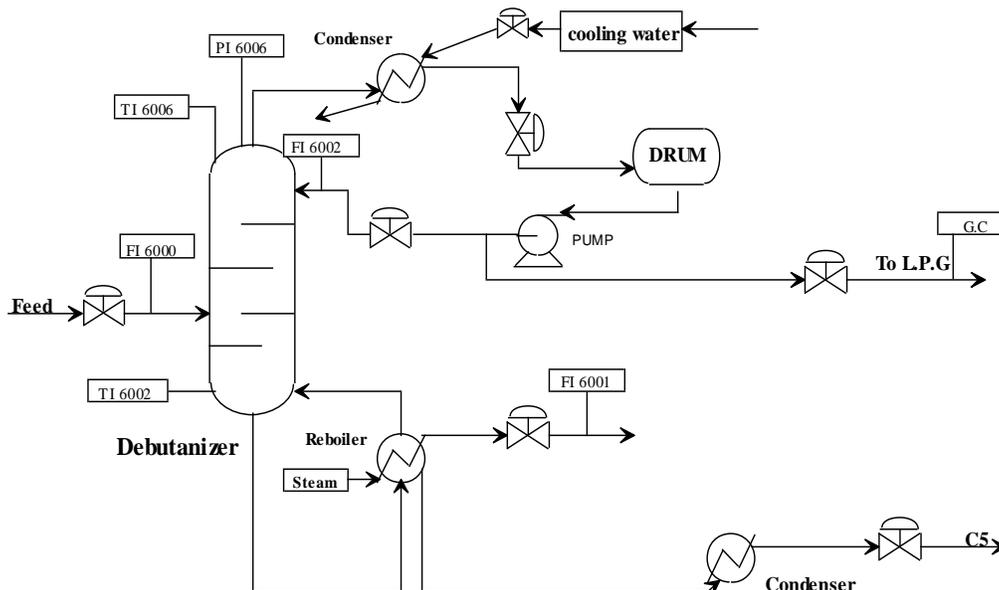
Figure 2. Schematic diagram of debutanizer column
