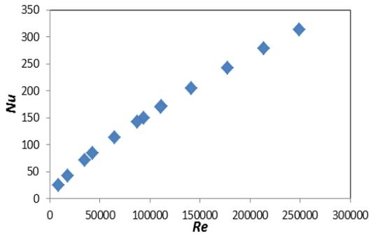
Fig-7: Experimental values of Nusselt number, by using Eqn. (4)
