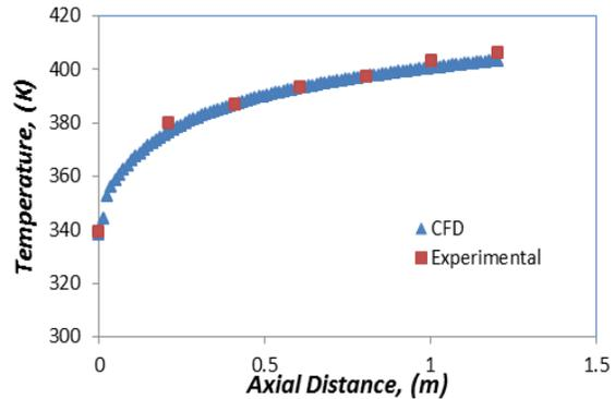
**Fig-5:** Comparison of the pipe wall surface temperatures between Experimental and CFD data
