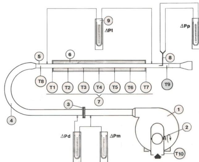
**Fig-1:** Experimental facility: (1) centrifugal blower; (2) damper; (3) flow meter (orifice plate  $ID=40 \text{ mm}$ ); (4) steel pipe; (5) copper pipe; (6) heater; (7) thermocouples; (8) Pitot tube; (9) differential manometer
