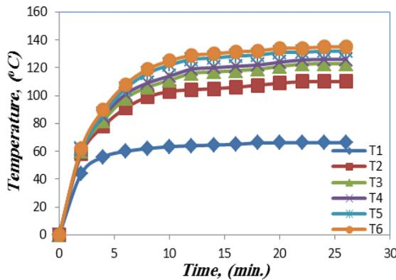
**Fig-3:** Wall temperature measured experimentally (Mass flux =68.797 kg/m<sup>2</sup>.sec, Re=1.1\*10<sup>5</sup>)
