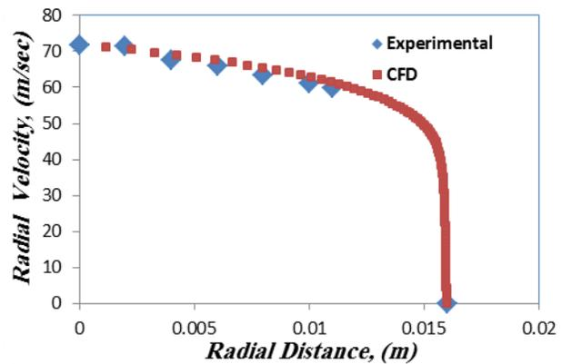
**Fig-6:** Comparison of radial velocity distribution for experimental and CFD data (Mass flux =68.797 kg/m<sup>2</sup>.sec, Re=1.1\*10<sup>5</sup>)
