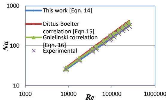
Fig-9: Comparison of  $Nu$  numbers as a function of Reynolds number for air
