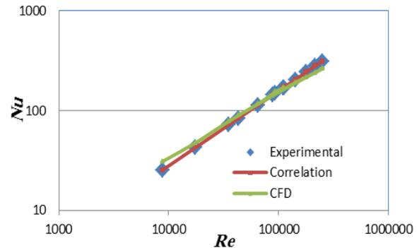
Fig-8: Comparison of Nusselt number for experimental, Correlation and CFD estimation
