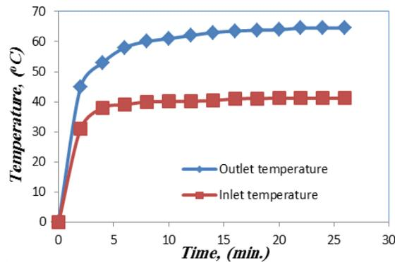
**Fig-4:** Temperature of bulk air measured experimentally (Mass flux =68.797 kg/m<sup>2</sup>.sec, Re=1.1\*10<sup>5</sup>)
