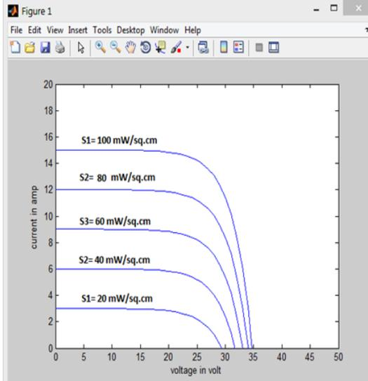
Fig 10 (a) I-V characteristics for different insolation values.
