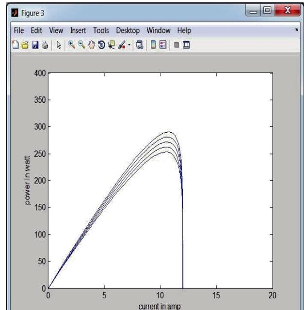
Fig. 7 P-I Characteristics of solar PV module at different cell temperature
