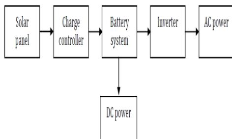
Fig. 1: Block diagram of a typical solar PV system
