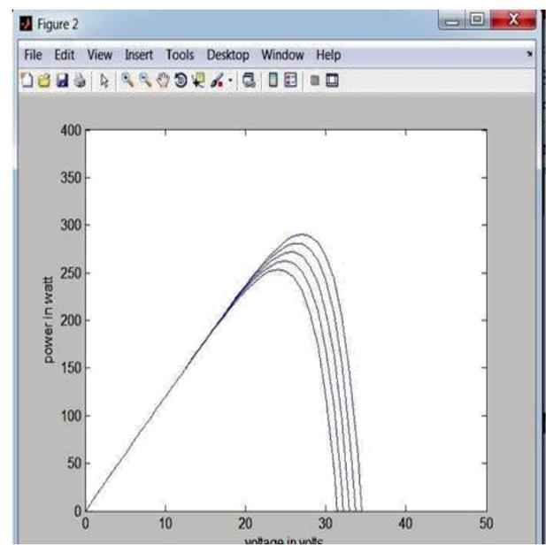
Fig 8 P-V Characteristics of a PV Module at different cell temperature
