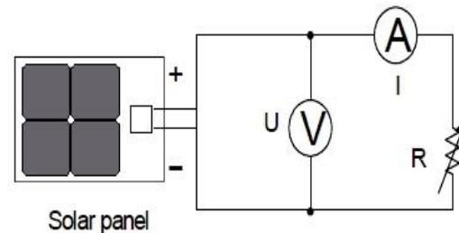
Fig. 2 Generalized panel equivalent circuit
