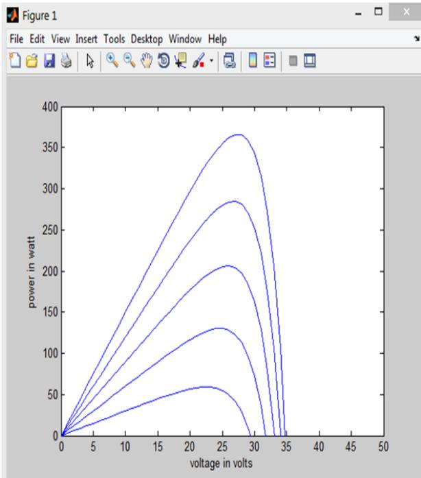
Fig. 5 P-V Characteristics of a solar PV Module at different insulation level.
