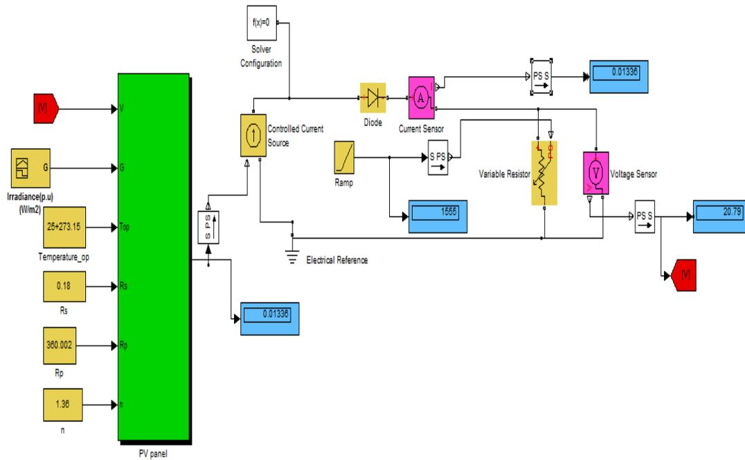
Fig 4: SIMULINK model of photovoltaic array
