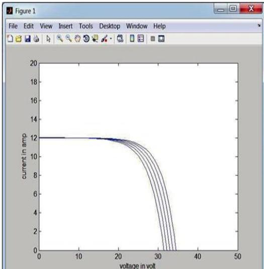
Fig 9 V-I Characteristics of solar PV module at different cell temperature.
