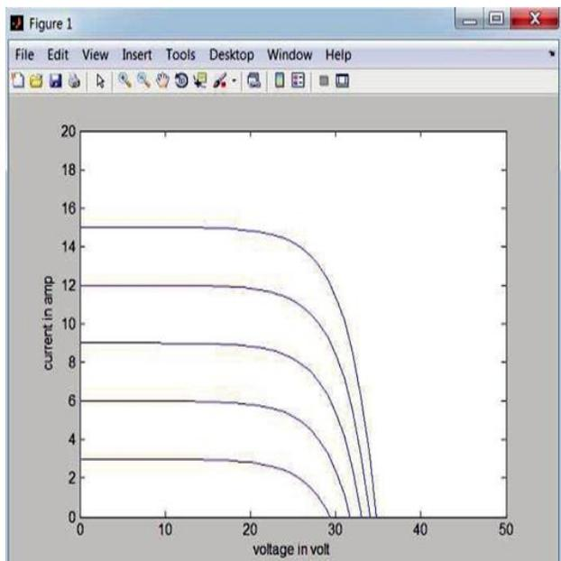
Fig. 6 V-I Characteristics of a PV Module at different insulation level.
