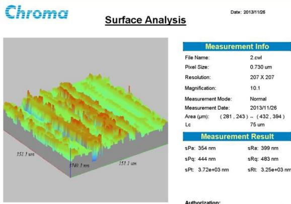
Figure 6(b) Ground surface of MIM AISI 316L workpiece of 2nd experiment under L9
