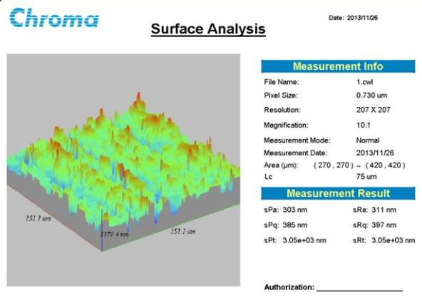
Figure 6(a) Ground surface of MIM AISI 316L workpiece of 1st experiment under L9
