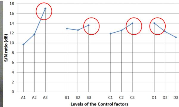
Figure 5 S/N ratio of L9 orthogonal table
