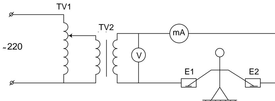
Fig. 1. The circuit determining the resistance of a person's body
