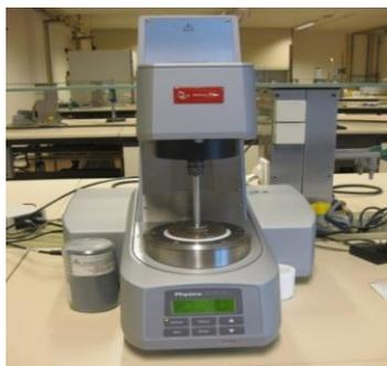
Picture 2. Reometer (Anton Paar Physica MCR 301) with spindle PP25
