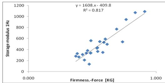
Figure 2. linear correlation of the Storage modulus 1Hz to the Firmness
