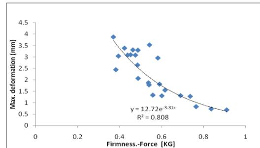
Figure 4. Exponential correlation of the maximum deformation to the Firmness
