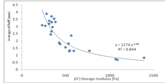
Figure 3. Exponential correlation of the maximum deformation to the Storage modulus
