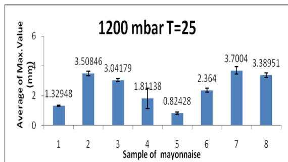
Figure 5. Maximum deformation (puff 1) for eight different batches of mayonnaises as measured with the FPD. The test displayed here were conducted at 7<sup>o</sup>, 19<sup>o</sup>, 25<sup>o</sup>C.
