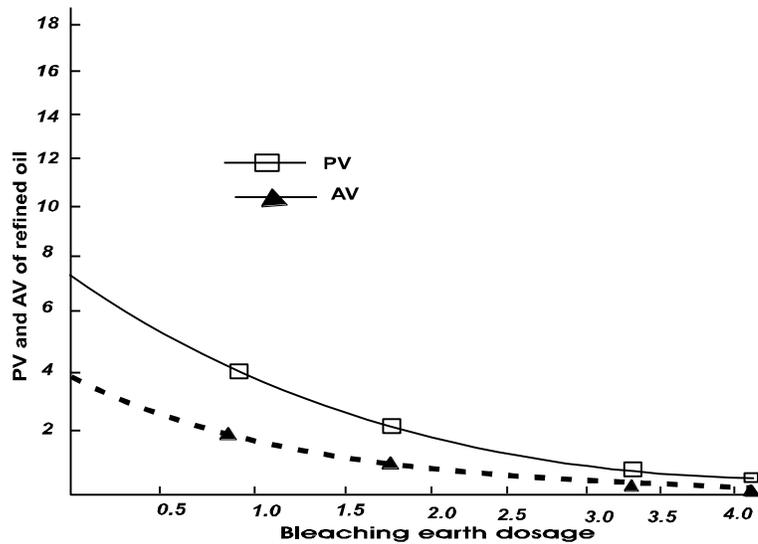
Fig 4 Reduction of PV and AV at increase earth dosage.
