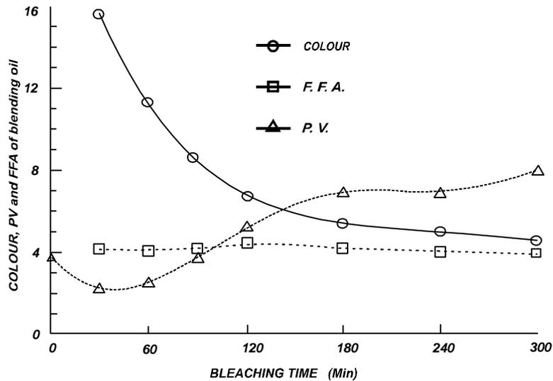
Figure 5 The effect of extended bleaching times on colour, p.v. and f.f.a. of bleached palm oil.
