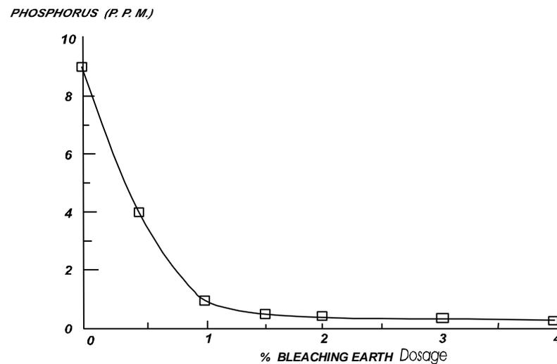
Figure 3 The effect of earth dosage on the phosphorus content of physically refined palm oil. Peroxide value and AV are reduced by increasing earth dosage, in a similar way as increasing bleaching temperature, Fig 4. However, and as shown in table 4, while PV is significantly reduced at the bleach temperature, AV is sharply increased from a temperature of 110<sup>0</sup>C.
