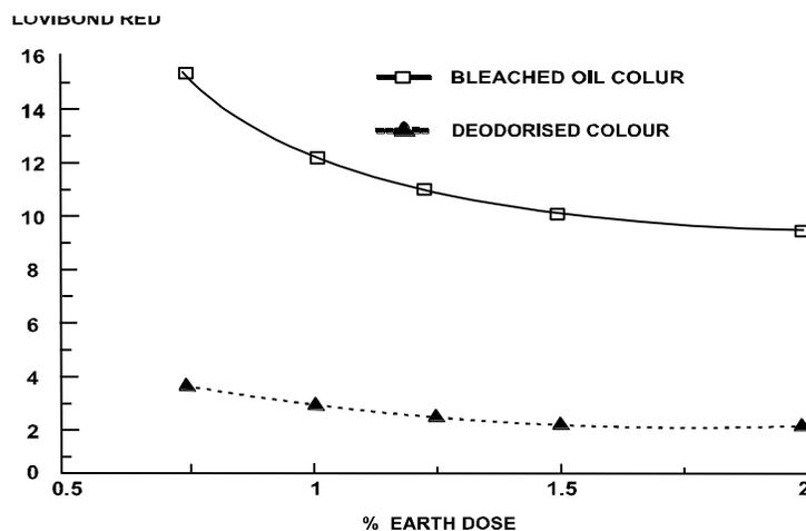
The deodorized colour, however, reaches a minimum between 1 and 1.5% clay dosage. There is no necessity to increase bleaching earth beyond 1.5% as this would produce no effect on the colour. The exact level of bleaching earth required will depend on the quality of the oil, and on the adsorptive power of the bleaching earth.
