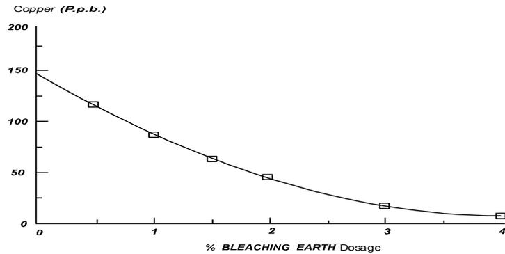
Figure 2 The effect of earth dosage on the copper content of physically refined Palm oil.
