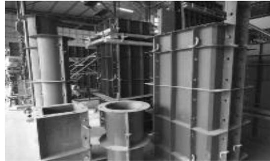
Fig. 2 Steel formworks
