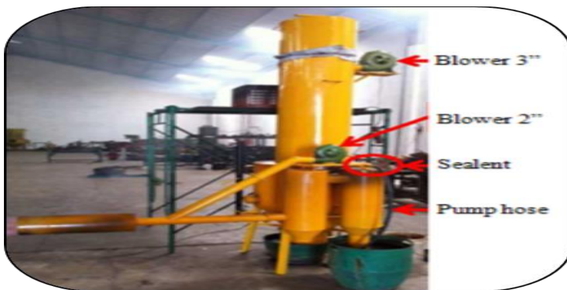
Figure 2. Prototype downdraft fixed-bed gasifier thermal 20 kW (rice husk) PT. ELCO
