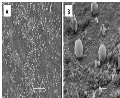
Figure 4. Micrographs of scanning electron microscopic (SEM) of ferric hydroxide colloids. A: scale bar 50  $\mu$ m, magnification 500. B: scale bar 5  $\mu$ m, magnification 1,500.
