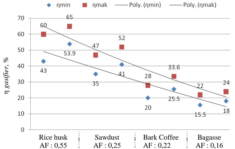
Figure 3. Correlation efficiency ( $\eta$ ) gasifier and air factor (AF)
