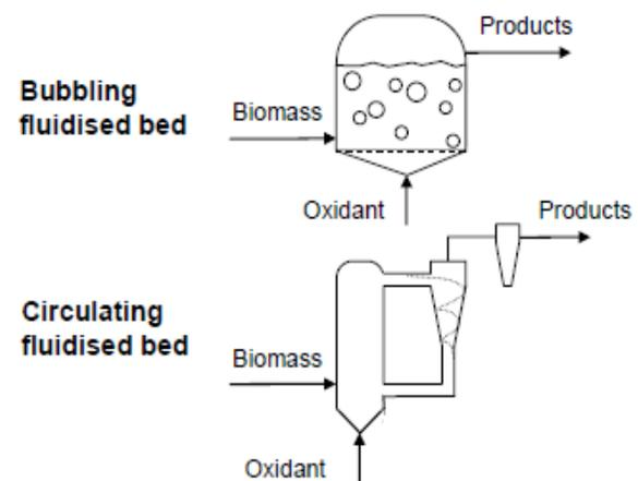
Figure 1. Differences in stream bed movement on fluidized-bed gasification system
