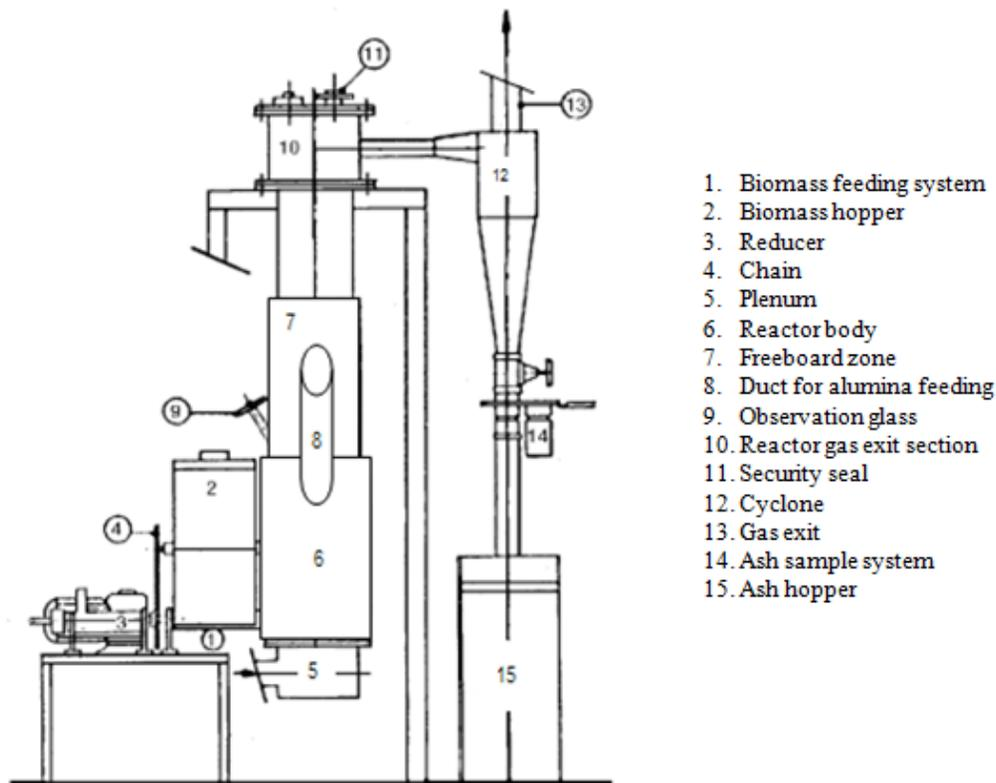
Figure 2. Experiment set-up for the biomass fluidized-bed gasifier
