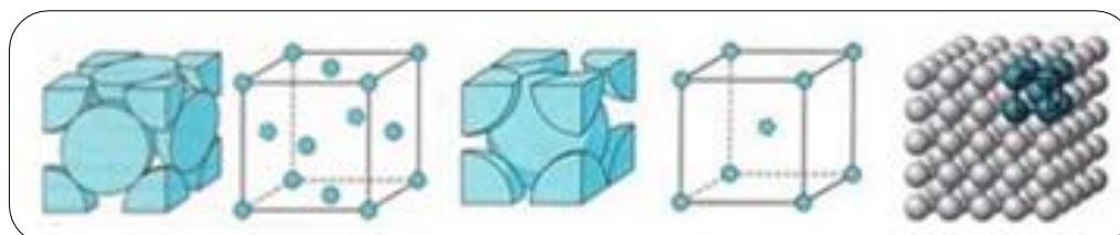
Figure 16. The crystal structure of faced centered cubic (FCC) dan body centered cubic (BCC)
