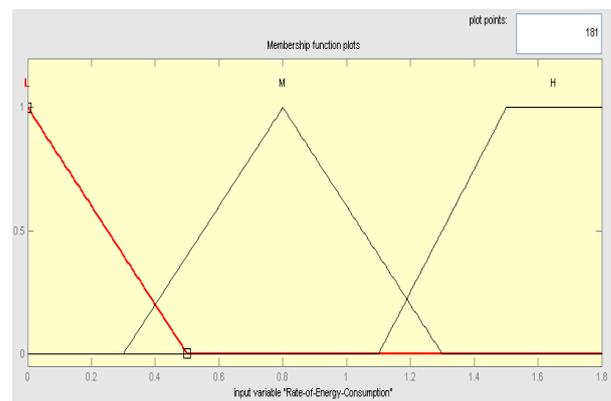
Figure 4. Energy consumption rate fuzzy membership function
