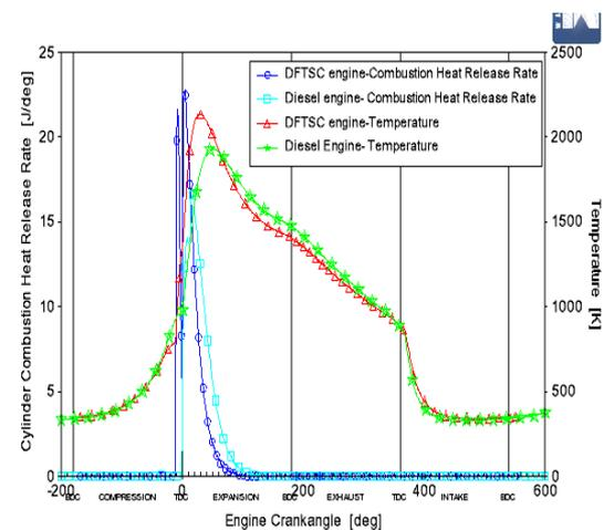
Figure 8. Cylinder combustion heat release rate Vs Engine crank angle for both engines at rated engine speed.
