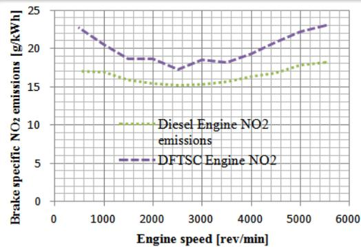
Figure 12. Brake specific NO<sub>2</sub> emissions Vs engine speed for Diesel engine and DFTSC Engine.
