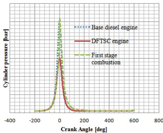
Figure 2. Cylinder pressure at the end of compression of baseline diesel engine and end of first stage combustion Vs crank angle
