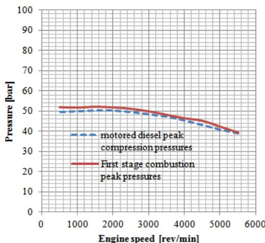
Figure 3. Peak compression pressure of the baseline diesel engine and the pressures at the end of first stage combustion of DFTSC engine Vs engine speed
