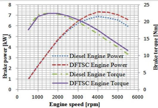
Figure 5. Comparison of brake power and torque Vs engine speed for both engines
