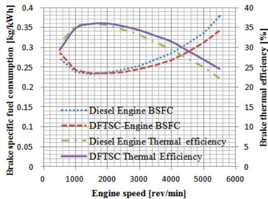
Figure 6. Brake specific fuel consumption and brake thermal efficiency Vs engine speed for both engines.
