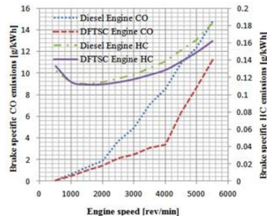
Figure 11. Brake specific CO emissions and brake specific HC emissions Vs engine speed for both engines
