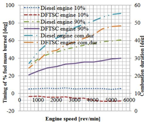
Figure 9. Timing of 10% and 90% fuel burned and combustion duration Vs engine speed for both engines.
