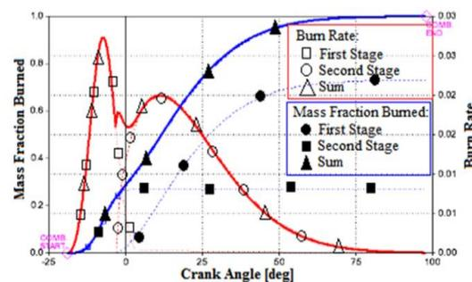
Figure 4. Mass fraction burned and the burn rate Vs crank angle for DFTSC engine
