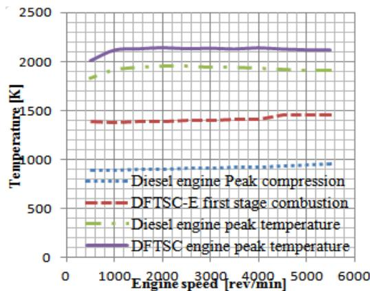
Figure 10. Peak compression and end of first stage combustion temperatures Vs engine speed for both engines
