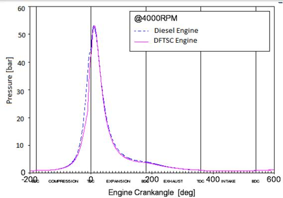
Figure 7. Cylinder pressure Vs Crank angle Diagram for both the engines at the rated engine speed.
