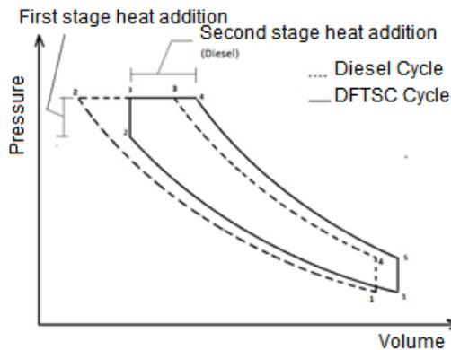
Figure 1. Ideal pressure – volume diagram representing Diesel cycle and DFTSC cycle
