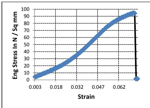
Fig.3: Stress-Strain Curve for sample C (with 5 % walnut kernel)
