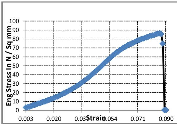
Fig 2: Stress- Strain Curve for Sample B (with 3 % walnut kernel)
