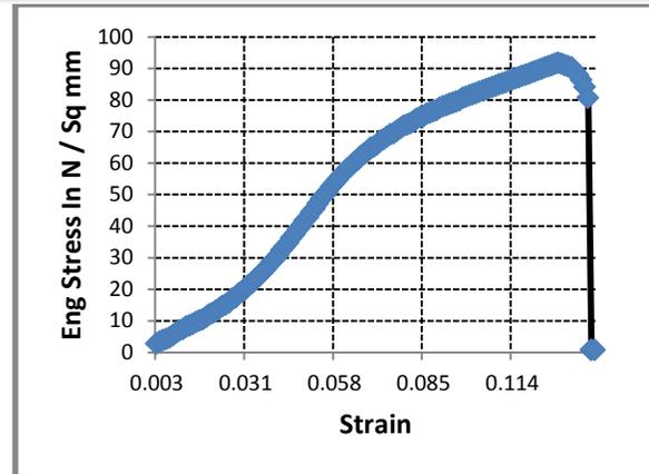
Fig.4: Stress- Strain Curve for Sample D (with 7 % walnut kernel)
