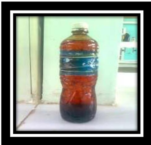
**C: Distillate obtained after pyrolysis**
