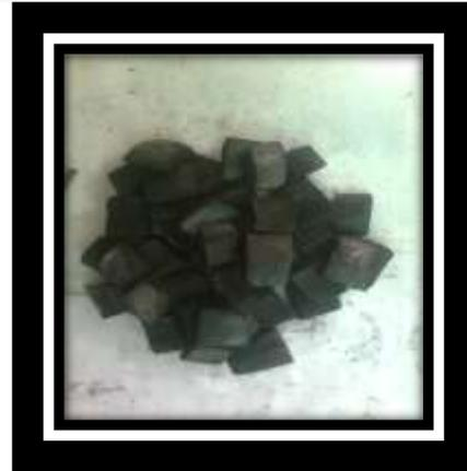
**B: Carbonized material after pyrolysis**
