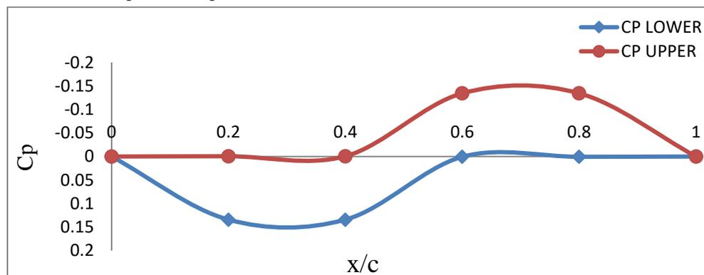
Figure 5: Pressure distribution for diamond shaped airfoil
