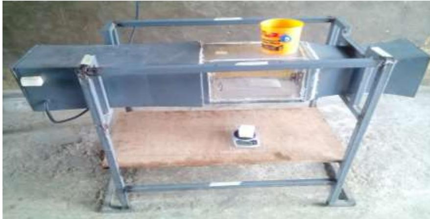
Figure 3: Picture of Indraft Supersonic Wind Tunnel
