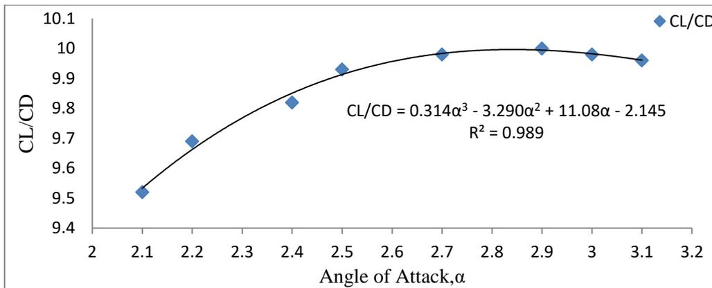
Figure 11: Variation of lift to drag ratio,  $(C_L/C_D)$ .with angle of attack,  $\alpha$ .
