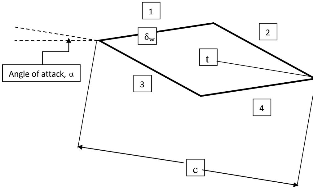
Figure 1: Symmetric diamond shaped airfoil.
