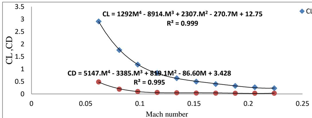
Figure 8: A typical graph showing variation of lift coefficient and drag coefficient with Mach number (Anderson, 2001).
