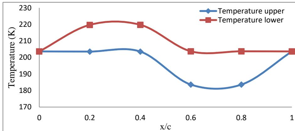
Figure 6: Temperature distribution for diamond shaped airfoil
