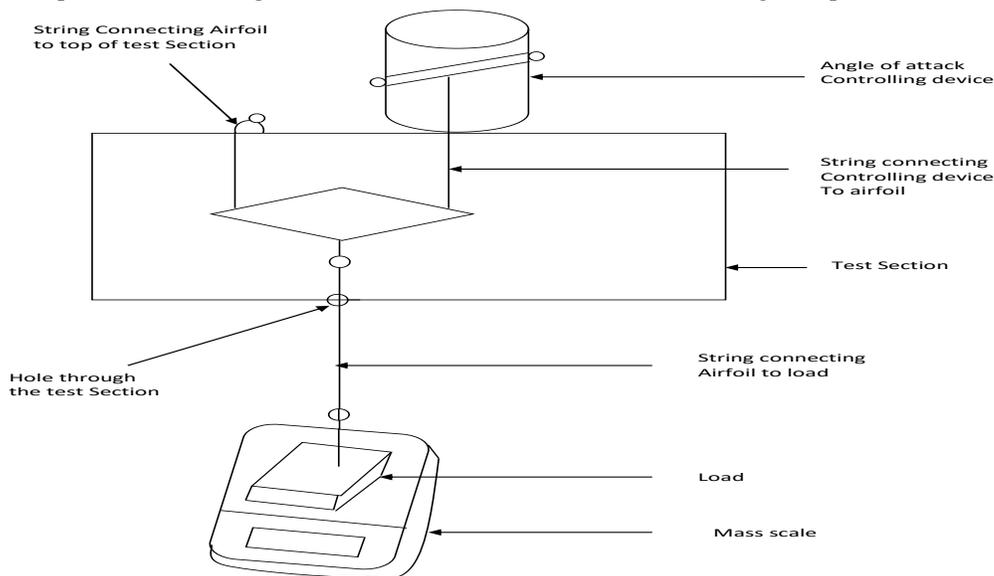
Figure 4: A sketch of diamond shaped airfoil connected to controlling device and load
