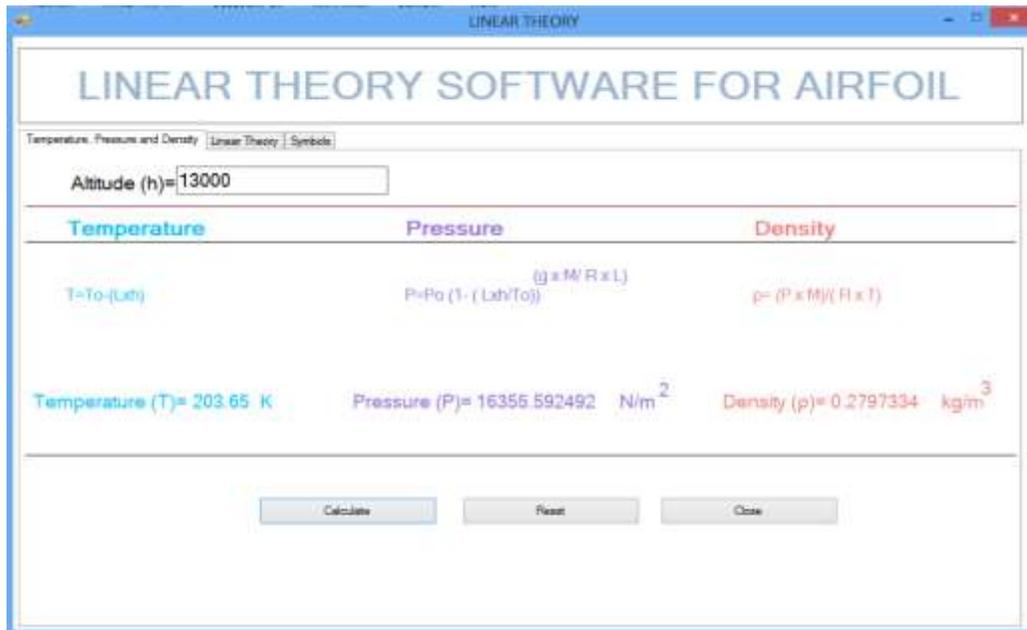
Figure 12: Acquisition of pressure, temperature and density data from linear theory software at a given altitude, h
