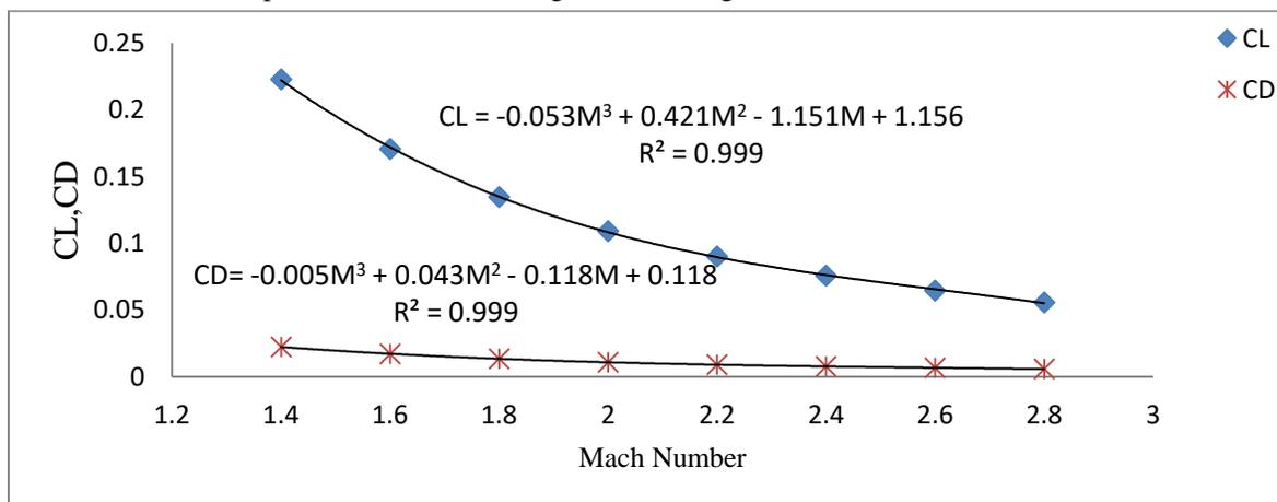
Figure 7: Variations of  $C_L$  and  $C_D$  with Mach number
