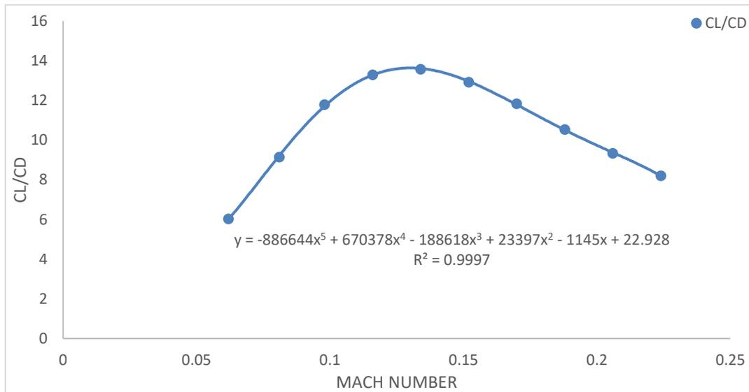
Figure 10: A typical graph showing variation of lift to drag ratio with Mach number (Anderson, 2001)
