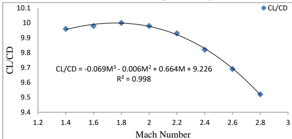
Figure 9: Variation of lift to drag ratio with Mach number
