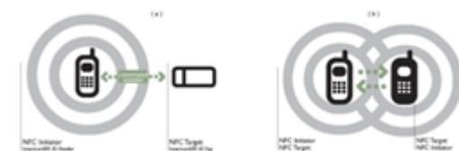
Figure 5. (a) NFC device emits an RF signal to activate a target (b) Two NFC devices establish an active communication between them [18].
