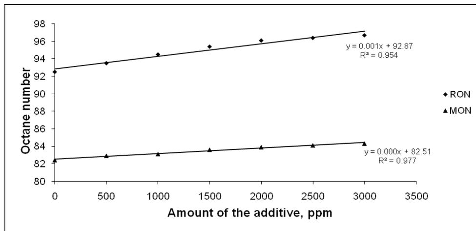
Fig. 2: Dependence of RON and MON of A92 gasoline (RON 92.5) on the concentration of the ferrocene antiknock additive
