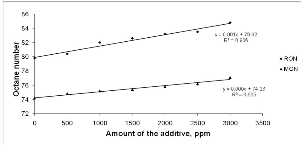
Fig. 1: Dependence of RON, MON of mixture A on the concentration of the ferrocene antiknock additive
