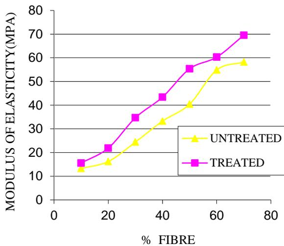
Figure 2: Effect of % Fibre on the Modulus of Elasticity of Untreated and Treated Bamboo Fibre - Reinforced Polyester Composite
