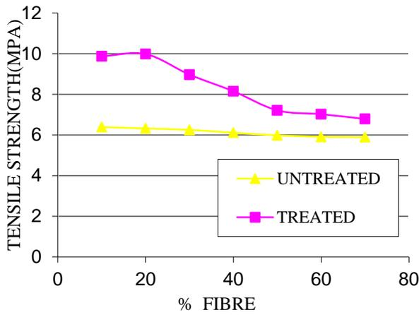
Figure 1: Effect of % Fibre on the Tensile Strength of Untreated and Treated Bamboo Fibre - Reinforced Polyester Composite
