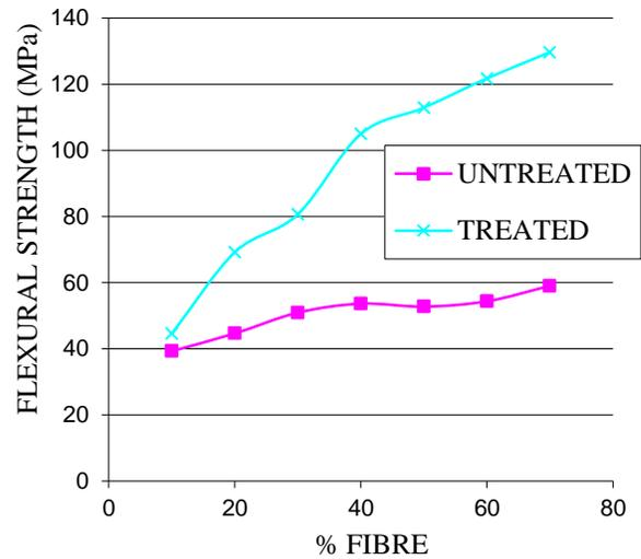
Figure 3: Effect of %Fibre on the Flexural Strength of Untreated and Treated Bamboo Fibre - Reinforced Polyester Composite
