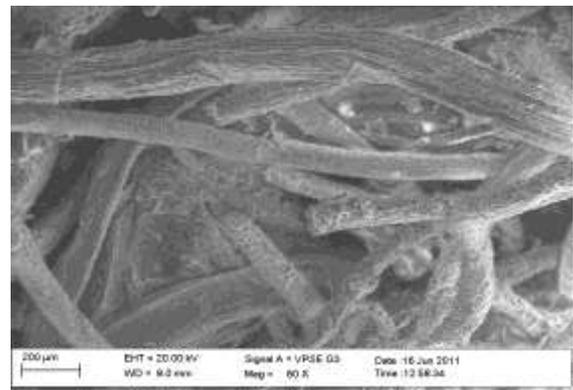
Figure 7: Fractured surface of a treated bamboo culm fibre composite showing fibre damage and little resin crack area.
