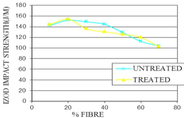
Figure 5 : Effect of %Fibre on the Izod Impact Strength of Untreated and Treated Bamboo Fibre - Reinforced Polyester Composite
