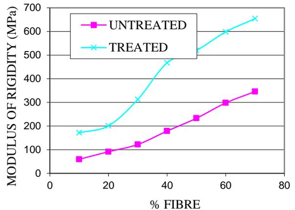
Figure 4: Effect of %Fibre on the Modulus of Rigidity of Untreated and Treated Bamboo Fibre - Reinforced Polyester Composite
