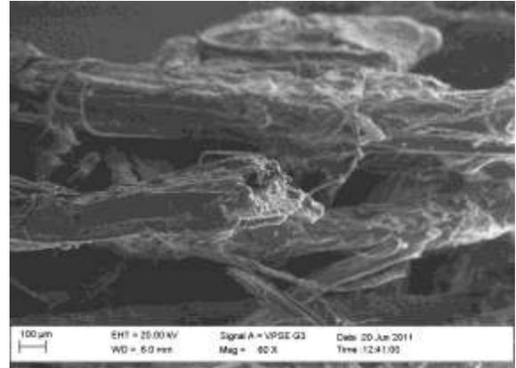
Figure 6: Fracture surface of an untreated bamboo fibre composite showing fibre peeling and large resin ‘crazing’.
