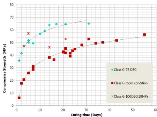
Figure 6. Compressive strength of Class G cement as a function of curing time
