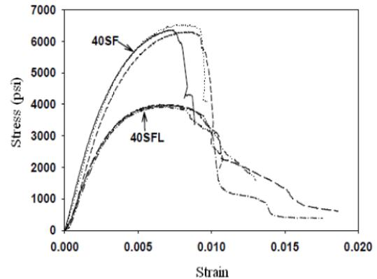
Figure 2. Uniaxial compression stress-strain curve at ambient temperature (Philippacopoulos and Berndt, 2001)
