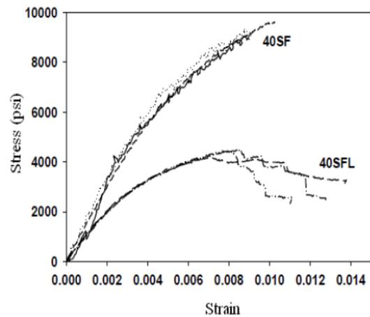
Figure 3. Uniaxial compression stress-strain curve at elevated temperature, (Philippacopoulos and Berndt, 2001)
