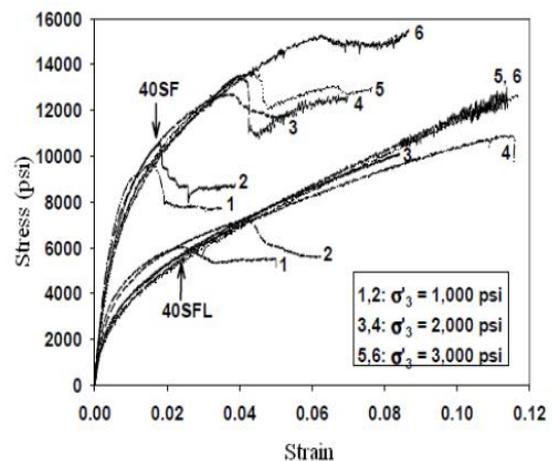
Figure 4. Triaxial compression stress-strain curve at elevated temperature, (Philippacopoulos and Berndt, 2001)
