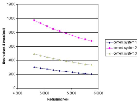
Figure 5. Equivalent stress in three cement systems, (Ugwu, 2008)
