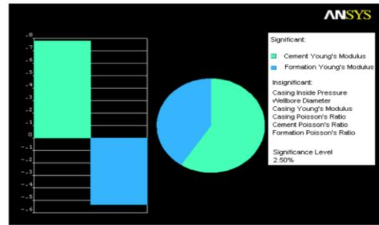
Figure 9. Cement maximum Von Mises stress sensitivity analysis, (Yuan et al, 2012)
