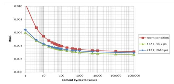
Figure 10. Cement Low Cycle Strain-N Semi Log Plots (the Confining Pressure of 4000 psi)
