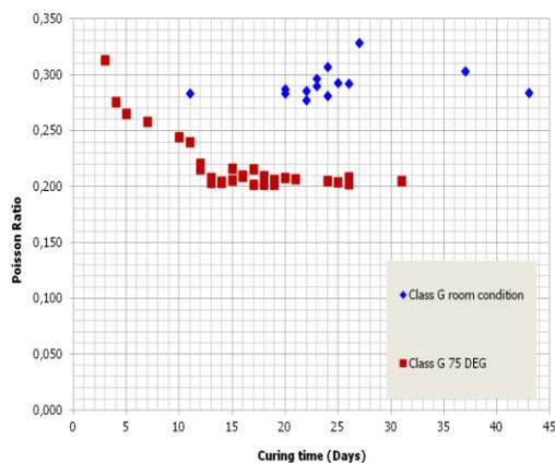
Figure 7. Poisson Ratio evolution of Class G cements
