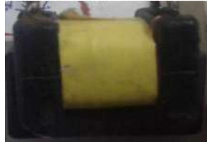
Fig. 20 Ferrite core transformer after designing
