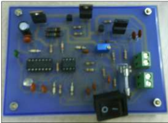
Figure 3. Circuit of solar charger controller in printed circuit board (PCB)
