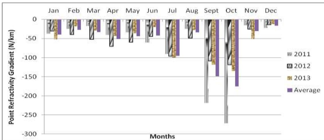
**Figure 1:** Monthly variation of point refractivity gradient in the lowest 100 m of the atmosphere not exceeded for 1% of an average year for Akure
