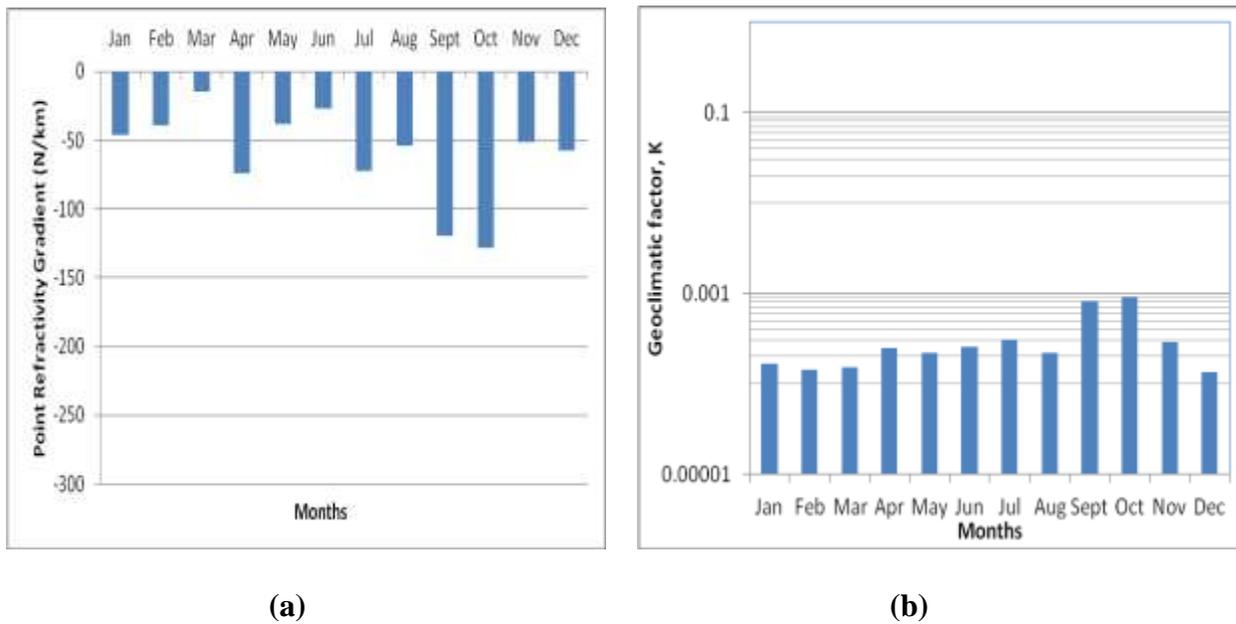
Figure 3: Seasonal variation of (a) point refractivity gradient in the lowest 100 m of the atmosphere not exceeded for 1% of an average year and (b) geoclimatic factor  $K$ .
