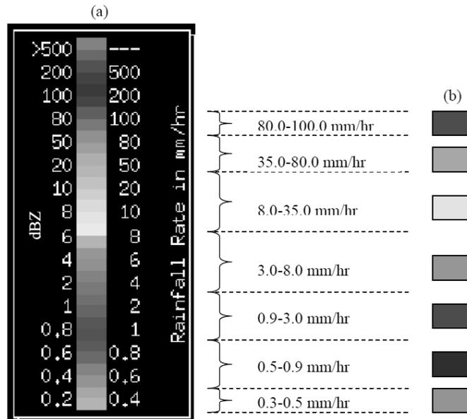
Figure 3. Various level of reflectivity colour derived from radar image (a) and simplified rainfall intensity colour after digitization (b)
