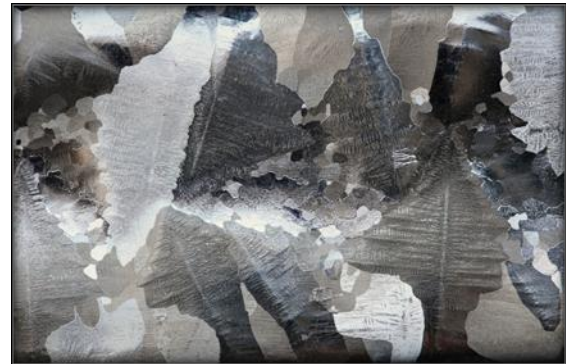
Figure 6: Aluminum bar surface etched [21]
