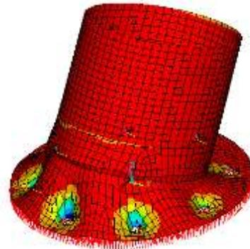
Figure 11: Contour of 3<sup>rd</sup> Principal Stress
