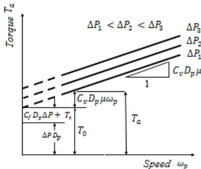
Figure 3. Applied torque vs. input speed
