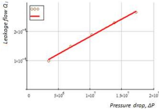
Figure 2.1 Graphically determined leakage flow vs. pump load pressure
