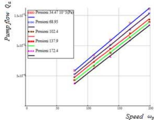
Figure 1.1 Measured flow rate vs. input speed
