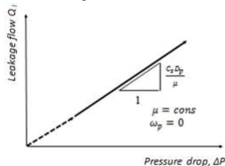
Figure 2. Leakage flow vs. pump load pressure
