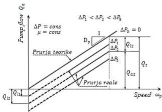
Figure 1. Flow rate vs. input speed
