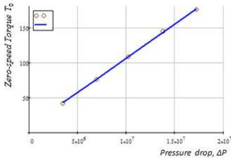
Figure 4.1 Graphically determined zero-speed torque vs. pressure drop
