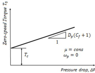
Figure 4. Zero-speed torque vs. pressure drop
