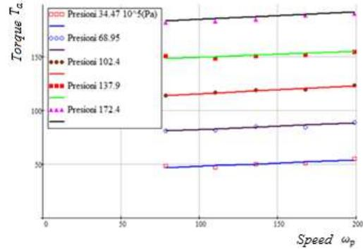
Figure 3.1 Measured applied torque vs. input speed
